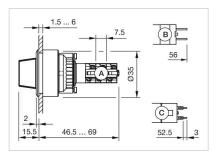
A = Solder terminal B = Plug-in terminal 2.8 x 0.5 mm C = Universal terminal 2.0 mm x 0.5 mm
