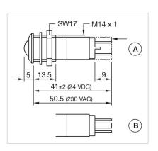
A = Protection tube (only 230 VAC) B = Tri-colour
