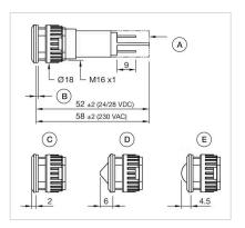
A = Protection tube (only 230 VAC) B = 1 gasket C = flat
