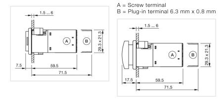
A = Screw terminal B = Plug-in terminal 6.3 mm x 0.8 mm
