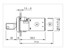
A = Screw terminal B = Plug-in terminal 6.3 mm x 0.8 mm
