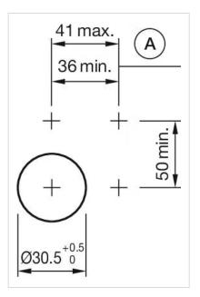
A = Action range of aligning pins
