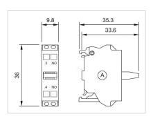
B = Spring-type terminal for Part No. 45-311.2Z40
