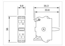
B = Spring-type terminal for Part No. 45-312.2Z40
