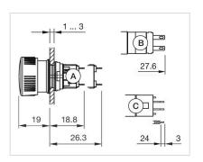
A = Solder terminal B = Plug-in terminal 2.8 mm x 0.5 mm C = Universal terminal 2.0 mm x 0.5 mm
