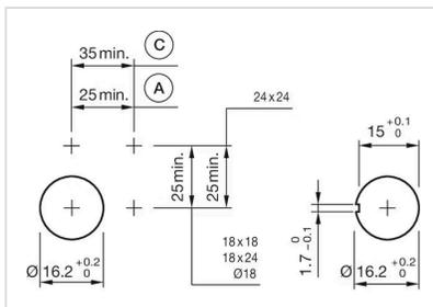
A = Solder/Plug-in terminal 2.8 mm x 0.5 mm
