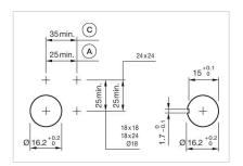
A = Solder/Plug-in terminal 2.8 mm x 0.5 mm
