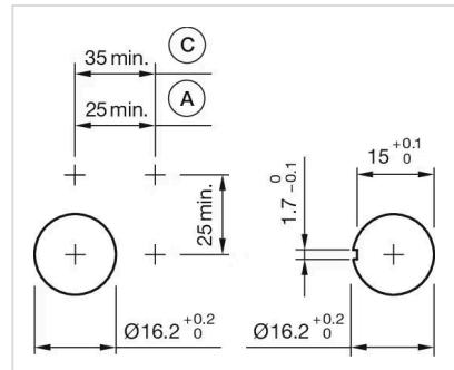
A = Solder/Plug-in terminal 2.8 mm x 0.5 mm
