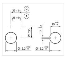
A = Solder/Plug-in terminal 2.8 mm x 0.5 mm
