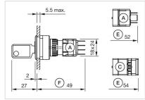
$\label{eq:Absolute} A = \mbox{Plug-in terminal } 2.8 \mbox{ mm x } 0.5 \mbox{ mm} \\ C = \mbox{Screw terminal}$
