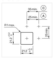
A = Solder/Plug-in terminal 2.8 mm x 0.5
