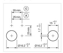
A = Solder/Plug-in terminal 2.8 mm  $\times$  0.5
