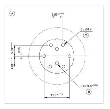
A = Drilling plan (component side) B = Positioning hole
