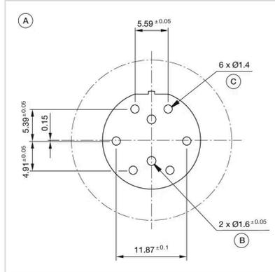
A = Drilling plan (component side)
