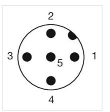
1 = NC 2 = LED+ 3 = Common 4 = LED-5 = NO A-Coded
