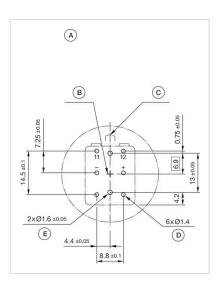
A = Drilling plan (component side)
