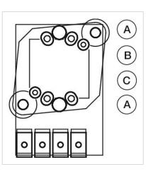
A = 4 = Switch  $B = x_{+} = LED$  Anode (+)  $C = 1x_{-} = LED$  Cathode (-)
