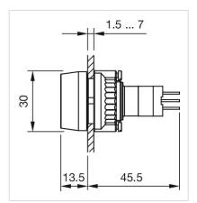
Pushbutton, Momentary, 250 V AC @ 3 A, 1 NC / 1 NO, Plug-in terminal, 2.8 x 0.5 mm, Round, Nature
