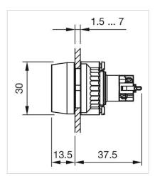
Illuminated pushbutton, Momentary, 250 V AC @ 3 A, 24 V AC/DC, 1 NC / 1 NO, Soldering terminal, Round, Yellow, Yellow
